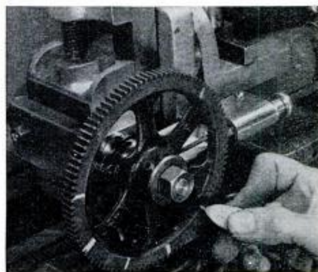
Gear wheel used as indexing head is chalk-marked into the number of divisions required by the work
